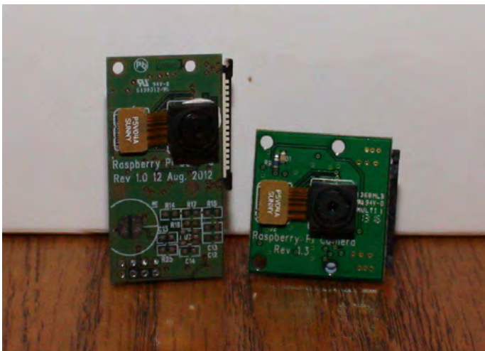
Prototype camera board (left) and final camera board (right)
