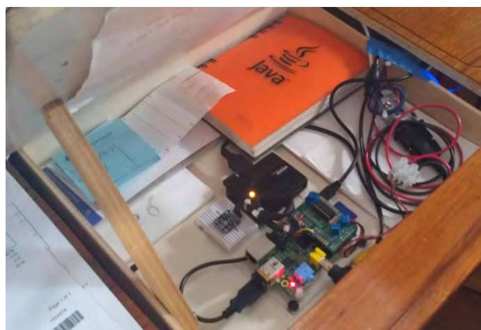
Raspberry Pi setup inside the chart table
