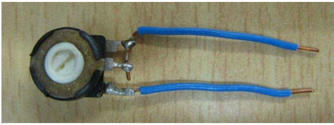
Fig. 2: The 1k potentiometer with the copper wires soldered to its pins.
