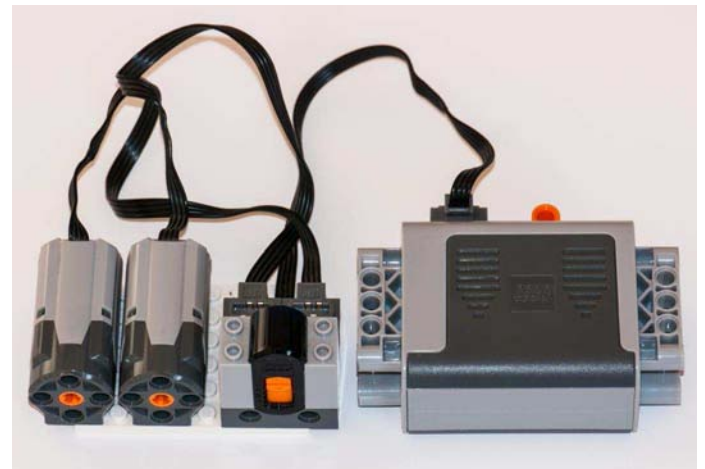
Figure 1 - Some LEGO® Power Functions components left to right: Motors, IR Receiver and Battery Box.
