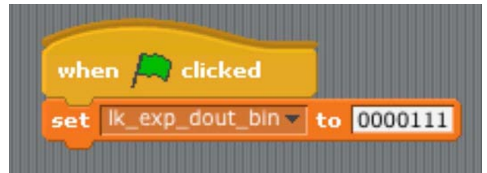
Figure 5.0 – Writing to the digital outputs in Scratch
