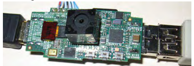
USB Stick sized early version of the Raspberry Pi
