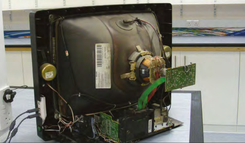
The wires from the Pi Zero are attached directly to the SCART board inside the TV
