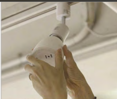
Below The Pi-powered sensor that necessitated the creation of the Pi Zero cluster board. It attaches to standard light fittings
