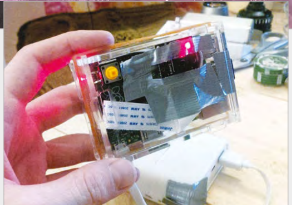
The mark two rig has a shutter button and LED to let you know when it's ready, although a preview screen will be added
