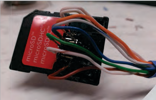
Left Mark interfaced directly with a microSD card converter to allow booting from the cartridge
