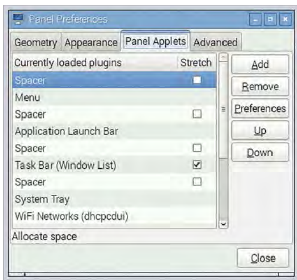
Right The Panel Applets tab on the Panel Preferences dialog allows plug-ins to be added, removed, and rearranged
