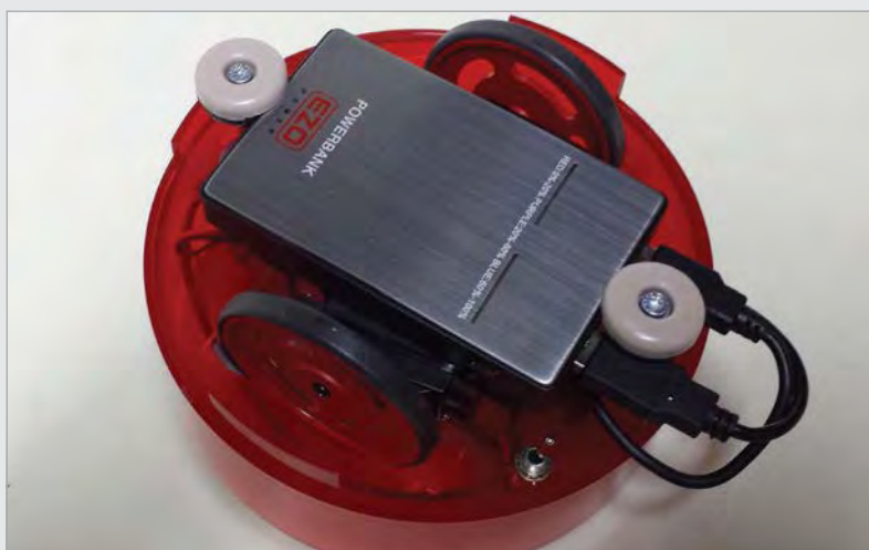
Above A standard smartphone battery pack is squeezed on top of the boards and inside the case
