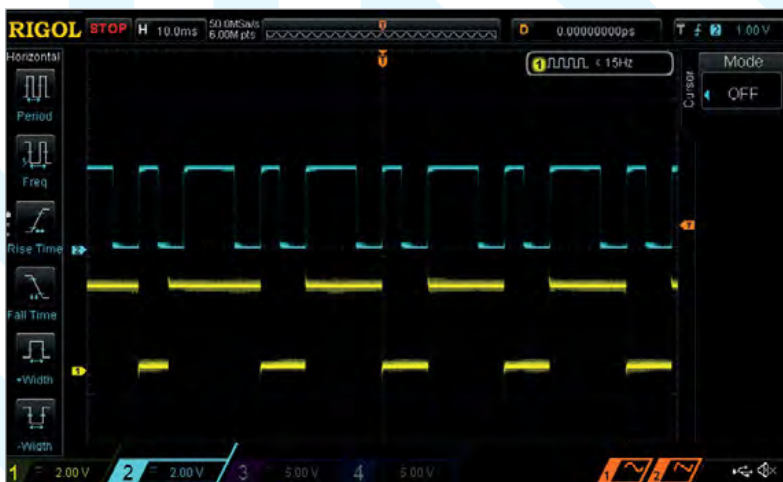
Figure 3 Oscilloscope trace showing the input pulse (top trace) and the GPIO output feedback (bottom trace)
