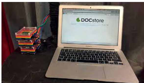
Above A cluster of four Raspberry Pis in a master-slave configuration hosts and executes SciBite's next-gen search tool
