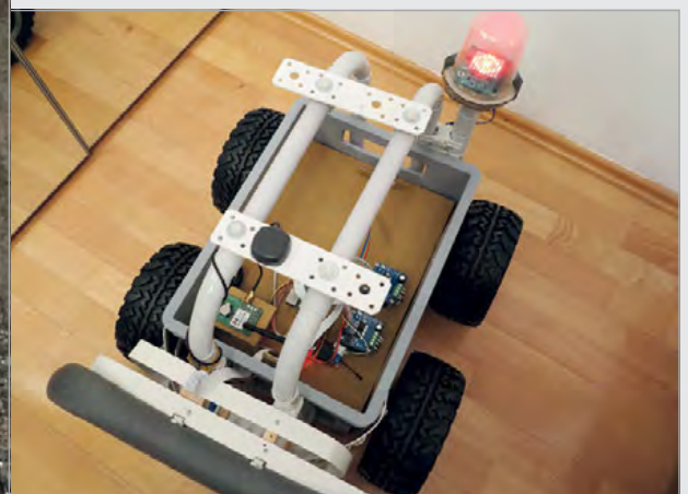
Below An early version of Big Rob showing the GPS system components, along with an illuminated Sense HAT at the rear
