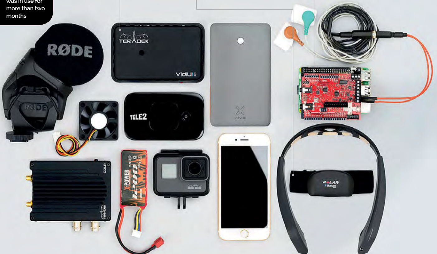
The Galvanic Skin Response Sensor, Polar Bluetooth HR monitor, and Muse headband all gather data on the emotional state of the wearer
