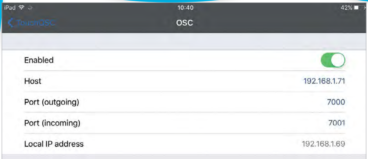
Fig 1: HOST: Set this to the address of the Raspberry Pi. Hover the pointer over the WiFi icon to find it. LOCAL IP ADDRESS: The address to put in the software is: String iPadIP = "192.168.1.69";
