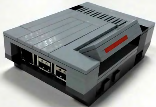
Putting the parts together results in this Raspberry Pi case. It looks like a classic NES console, but with access to the Raspberry Pi ports. The lid (used for cartridges in the original NES) provides access to the GPIO pins
