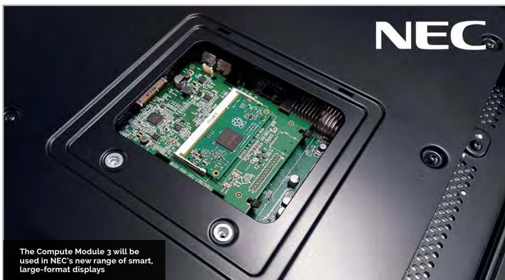
The Compute Module 3 will be used in NEC's new range of smart, large-format displays
