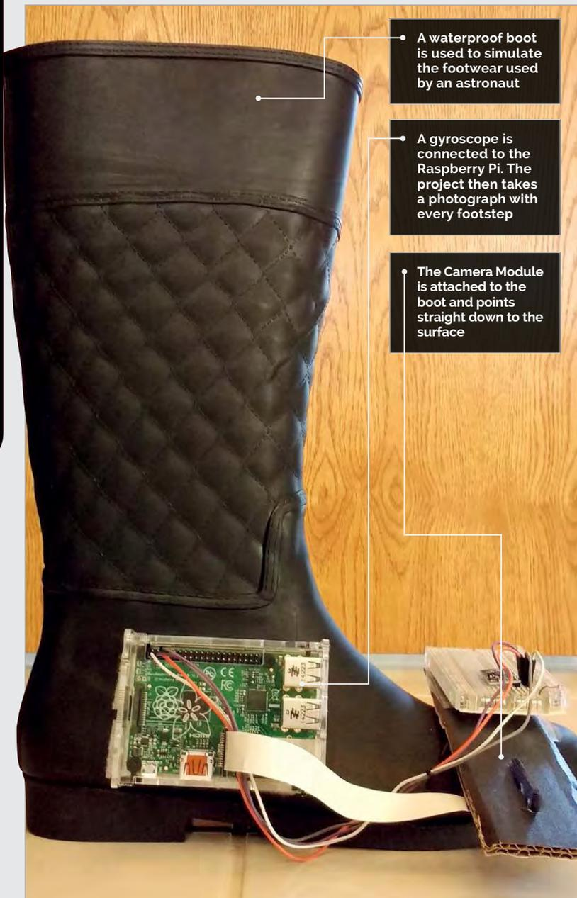
A waterproof boot is used to simulate the footwear used by an astronaut
