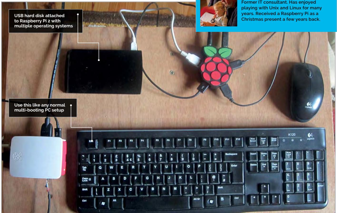
USB hard disk attached to Raspberry Pi 2 with multiple operating systems
