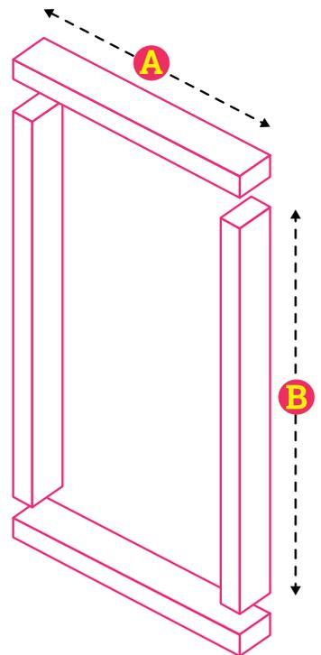
**A** Width of monitor + depth of wood x 2
