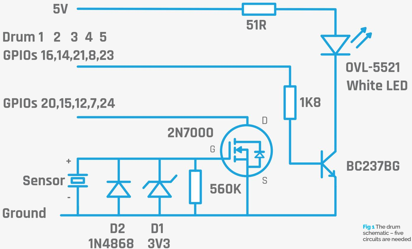
Fig 1 The drum schematic – five circuits are needed
