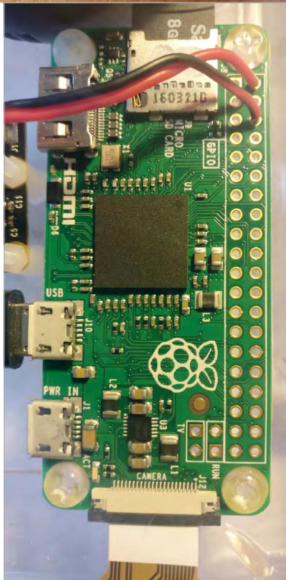
**Left** Connection from the output of the UBEC to the Pi's 5V and GND GPIO pins
