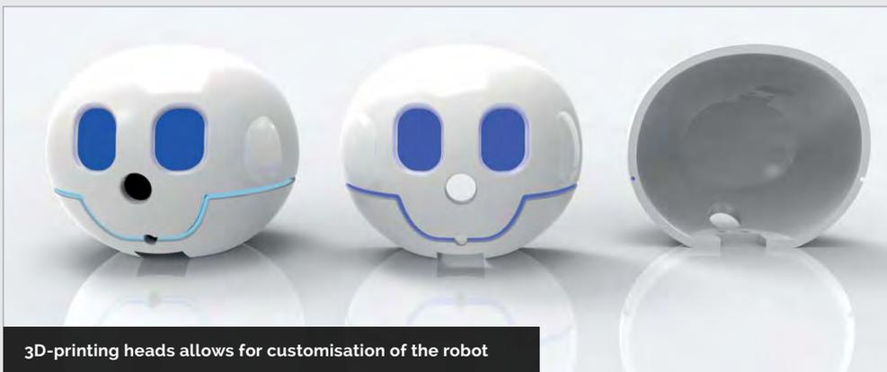
3D-printing heads allows for customisation of the robot
