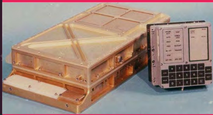
The AGC computer and its control pad. Computers were very different in the Sixties, relying mostly on magnetic ribbon for storage
