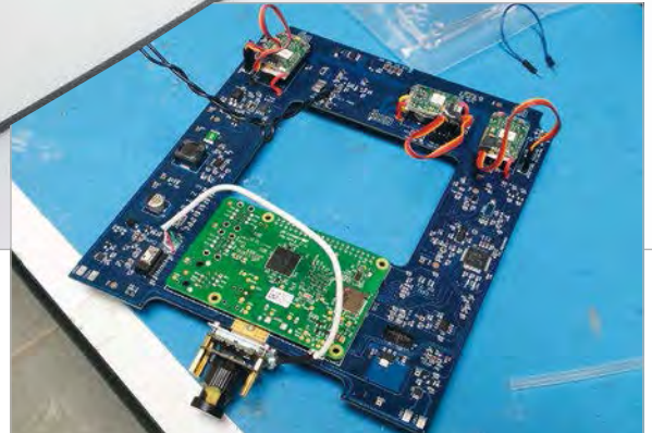
The bare-bones motherboard connects to the Raspberry Pi 3 at the front, which in turn controls much of the craft
