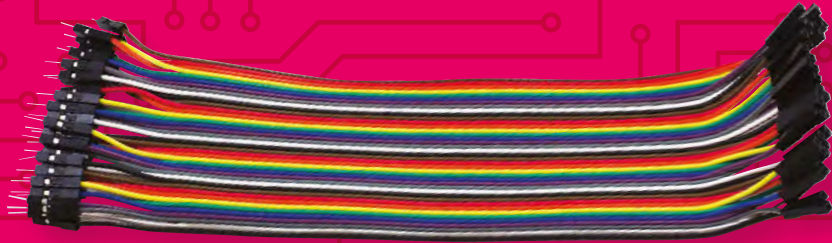
Jumper wires are useful for connecting to the GPIO pins
