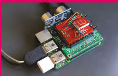
The project in action; the Pi is measuring how far it is to the Raspberry Pi 3 box.
