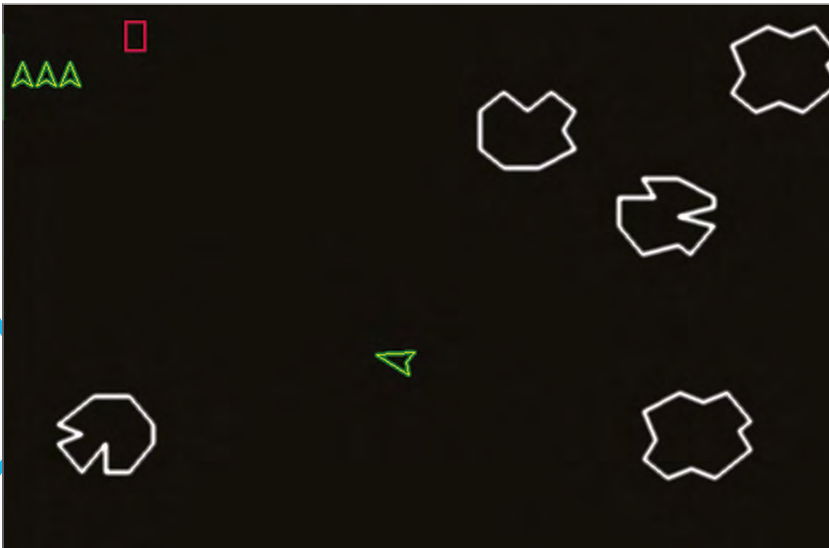
Left The code takes your ship's orientation into account using trigonometry, so that bullets can be fired in the correct direction
