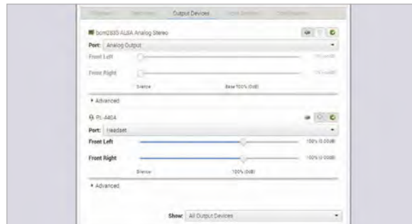
Left PulseAudio offers better control of the audio output to the Bluetooth device than the defaults
