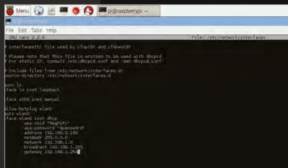
Above To set a static IP on the desktop interface, you'll have to go through the same process
