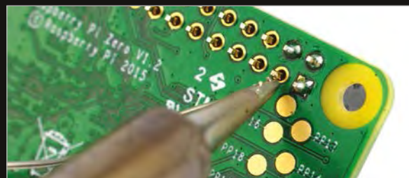
Above Take your time when soldering the pins, and be careful not to connect two or more together with excess solder
