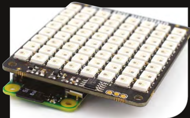
Left The small size of the Pi Zero means it's hidden away entirely underneath most HATs, making for a compact build
