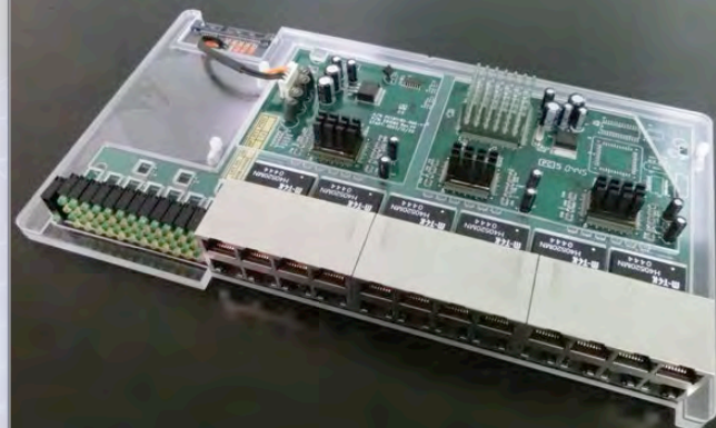
The bottom section of David's cluster consists of two 24-port switches
