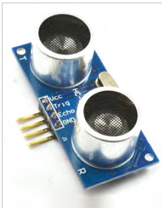
Left The HC-SR04 Ultrasonic Rangefinder. Cheap-as-chips sonar
