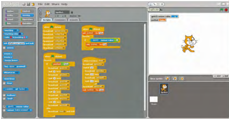
Left: Four pieces of code are used for GPIO configuration, light sequence, button press detection, and buzzer beeping
