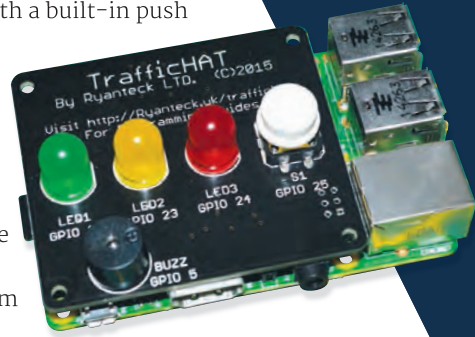
Above The Traffic HAT features LEDs, along with a button and buzzer
